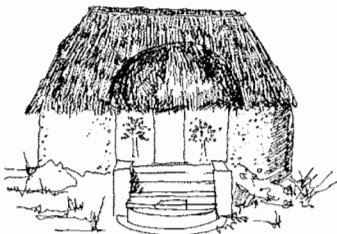
ADOBE HUT (mud and thatch)
